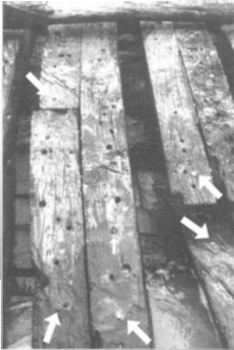
Figure 9. Planks possibly from bottom of hull, with a few Muntz metal (larger arrows) and tree nail (smaller arrow) fasteners left.
