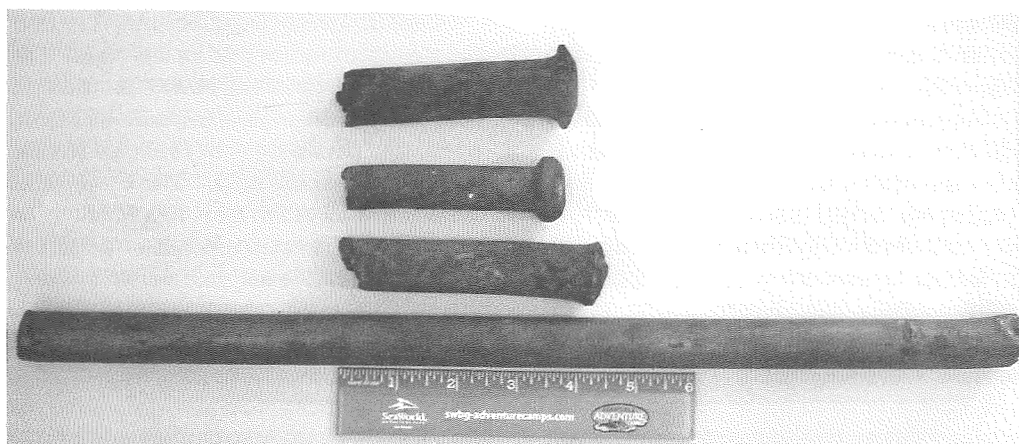
Figure 11. Muntz metal fasteners on display at ANERR education center (scale in inches). Photo by Erik Lovstrand.
