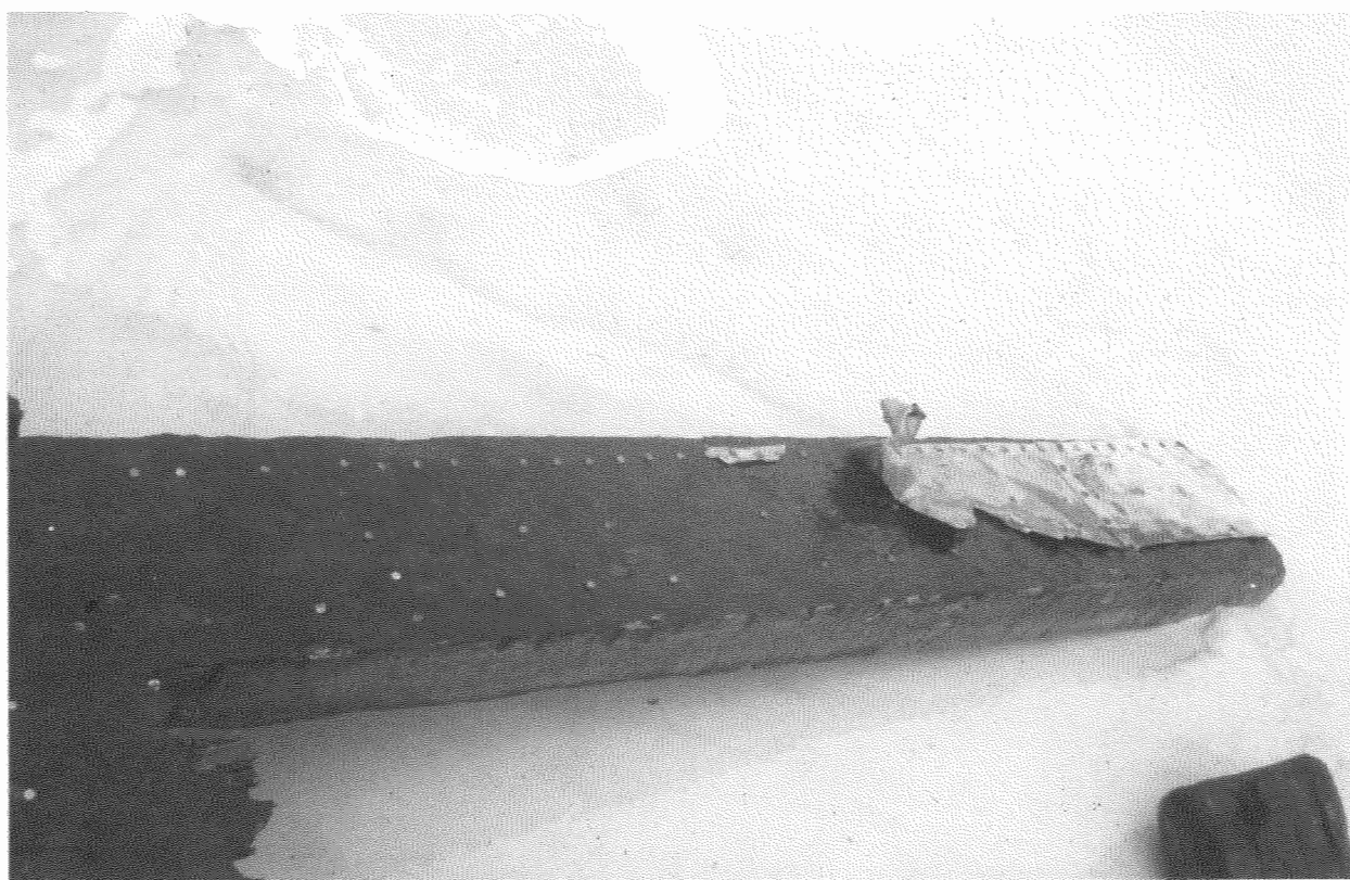
Figure 6. Closeup of only hull plank to retain copper sheathing, curled up on the edge; also visible are round heads of copper and Muntz metal fasteners (nails or spikes). View facing northwest. This plank is the one extending farthest to the left in Figure 4.5
