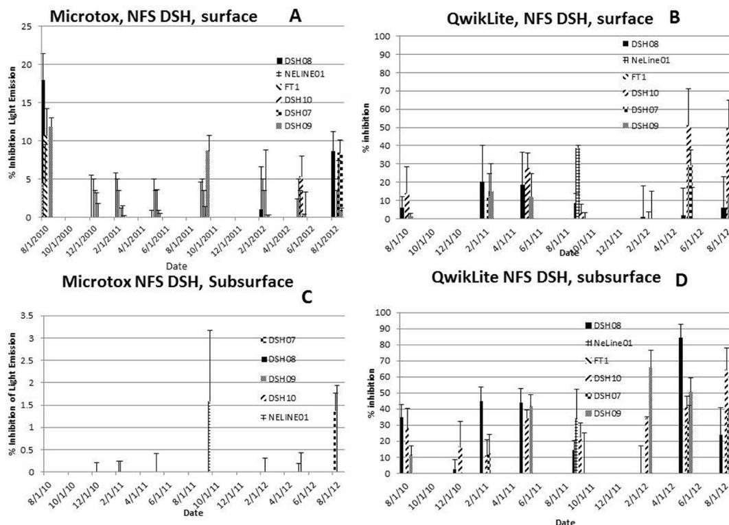
**Figure 3.** Long-term monitoring of surface waters from the NEGOM including Stations DSH07–DSH 10, NELINE01 and FT1. Error bars are actually  $\pm$  range of true replicates. Where error bars appear at zero % light inhibition indicates the magnitude of the range between replicates that averaged a zero response. Microtox (A) surface and (C) subsurface samples. Results of QwikLite analyses of (B) surface and (D) subsurface samples.
