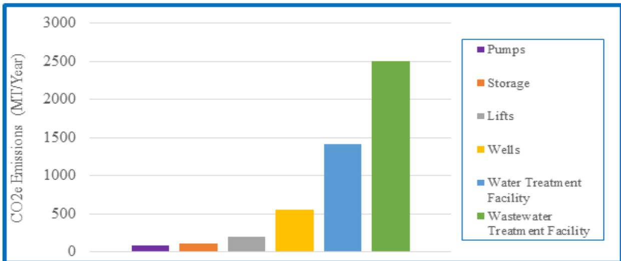
Figure 7. 2017 CO<sub>2</sub> Equivalent Emissions from Water Transfer Components
