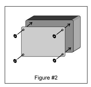
Replacing the upper lamp requires removal of the lamp housing. Remove the two screws which hold the housing in place. Observe the same warnings as shown above when handling the lamp. Replace the lamp and lamp housing.
