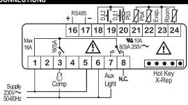
Supply: 120Vac or 24Vac: connect to terminals 5-6. The X-REP output is optional
